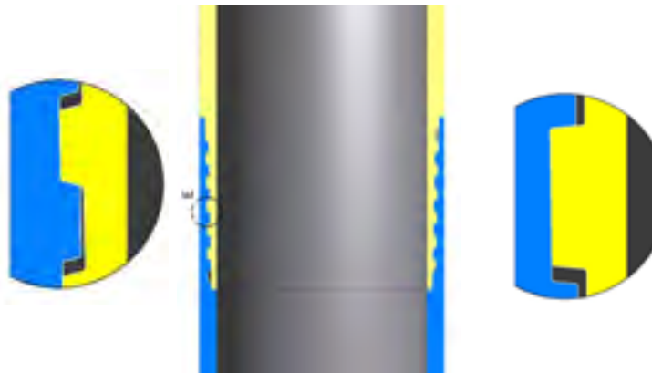
Thread profile of ATW, BTW & NTW rods.
